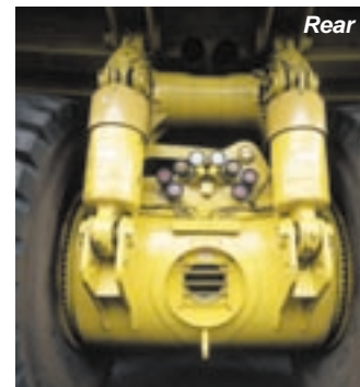
Nitrogen gas/oil damping suspension design
